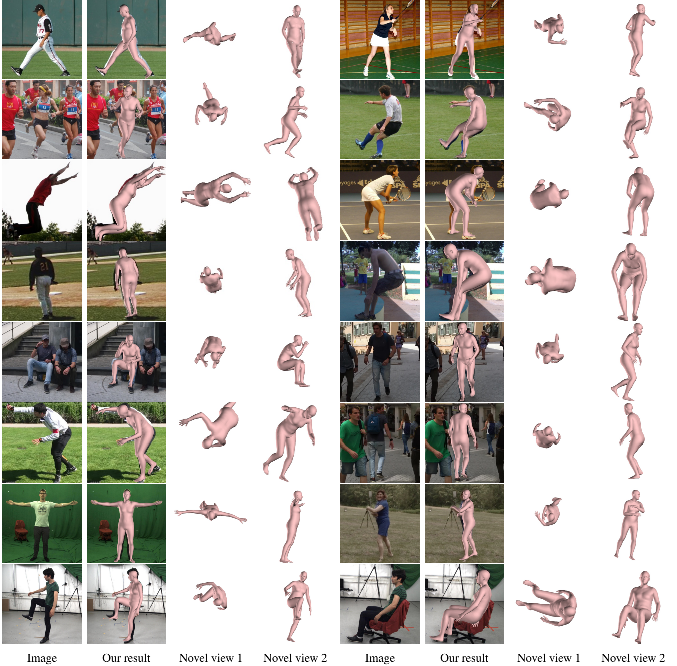
Figure 1: Successful results of SPIN. For each example from left to right: Image, Our reconstruction result in the camera frame, Our reconstruction result from a novel view (top view), Our reconstruction result from a novel view (side view).
